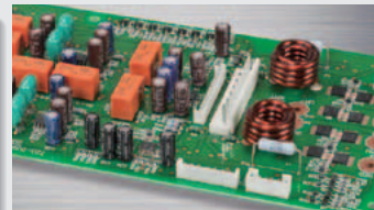
Protection and meter circuit assembly
