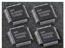
AK4490EQ delta-sigma type D/A converter chips
